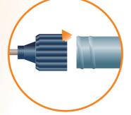
**B** Unscrew and remove delivery tube end of the Dryzone application gun
