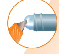
D Cut and remove the visible end of cartridge to prevent foil and sealing ring blocking the Dryzone delivery tube.
